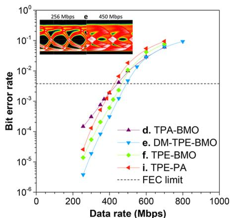
**Figure 4.** BERs versus data rates of the AIEgens measured at an incident power of  $P_i = 6.12$  mW using OOK. The forward error correction (FEC) limit is  $\text{BER} = 3.8 \times 10^{-3}$  (dashed line). The eye diagrams of DM-TPE-BMO at 256 and 450 Mbps are inserted.
