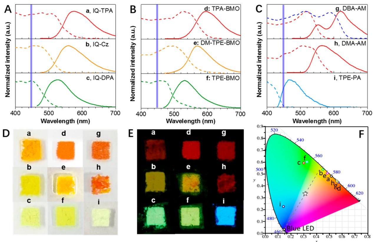
**Figure 2.** (A–C) Normalized excitation and emission spectra of the AIEgens in solid state. The vertical blue lines show the 450 nm excitation of the blue laser diode (denoted as LD, whose wavelength is same as the blue LED chip). (D) Bright-field photo of the AIEgens in solid state. (E) Dark-field photos of the AIEgens in solid state under the 365 nm excitation of UV analyzer. (F) CIE coordinates of the AIEgens generated on CIE 1931 chromaticity diagram according to their emission spectra.
