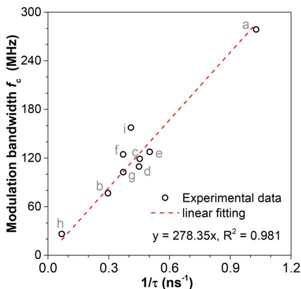
**Figure 5.** Plot of the relation between effective lifetimes  $\tau$  and modulation bandwidths  $f_c$  of these AIEgens. The red-dashed line is the linear-fit line of the scattered sample points with the intercept set as zero ( $f_c = k \times 1/\tau$ ).
