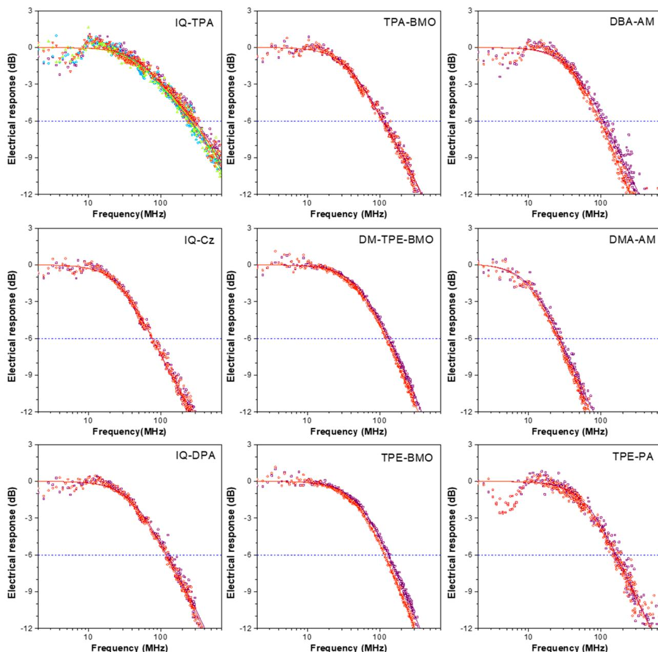
**Figure 3.** Plots of the electrical responses of these AIEgens versus frequency (scatter). The nonlinear fitting curves are performed with two-component model as shown in eq S19 (line). The modulation bandwidths  $f_c$  are calculated and averaged at  $-6$  dB electrical response.
