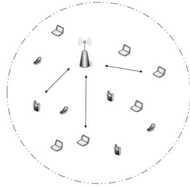
Fig. 4: A typical AP-Client topology in WLANs, with a maximum number of 15 clients randomly distributed.
