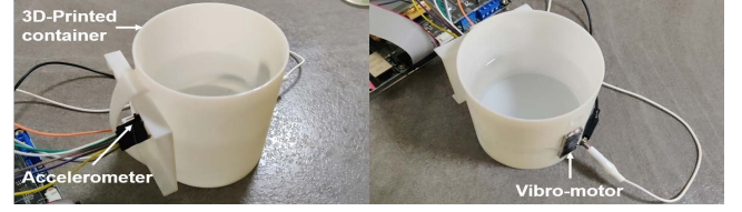
Figure 3: Confirmatory experiments were set up by separate motor, accelerometer, container and alternating current power supply.
